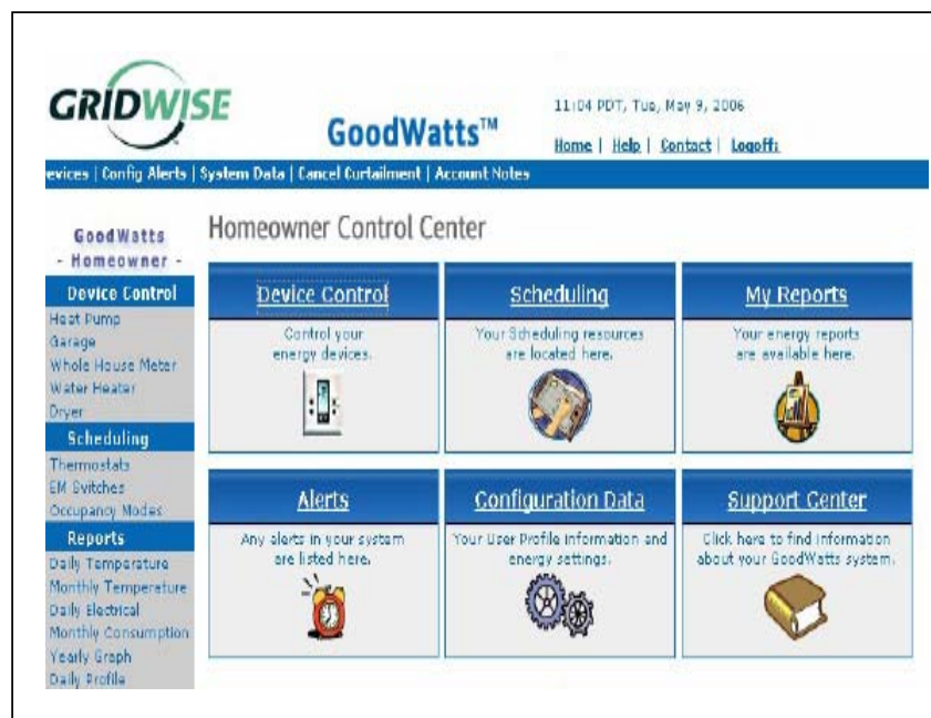
Figure 2: Consumers may be able to make their electricity choices via a simple point-and-Click Web interface, as in this example from a DOE GridWise demonstration project. Source: This graphic was produced at the Pacific Northwest National Laboratory under Contract DE-AC05-76RLO 1830 with the U.S. Department of Energy, and the GRIDWISE™ trademark is owned by Battelle Memorial Institute.
