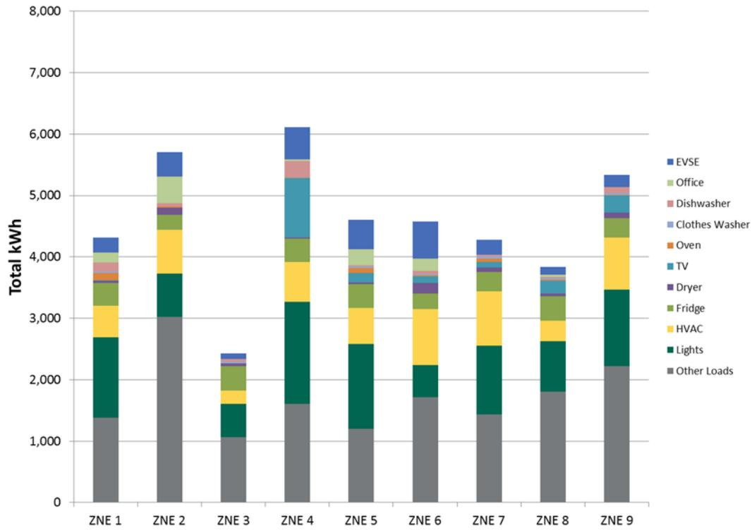
Figure 9: RESU Block Energy Use Breakdown (July 1, 2013 to February 28, 2014)
