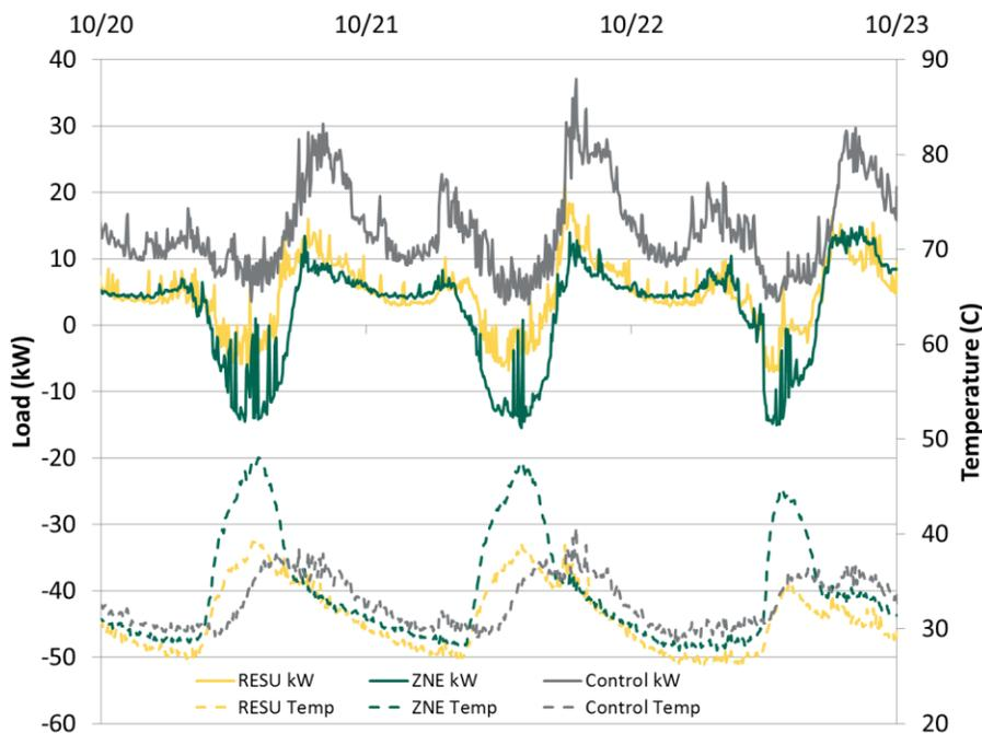
Both the ZNE and RESU Block transformers fed power back into the grid during peak solar periods. The Control Block transformer (10% PV penetration) showed reduced load during the day while the RESU Block (75% PV penetration) exported to the circuit during peak periods. The additional generation on the ZNE Block—which has 100% PV penetration—was readily apparent on the transformer, as the power output by the entire block during the test period was over 15 kW.
