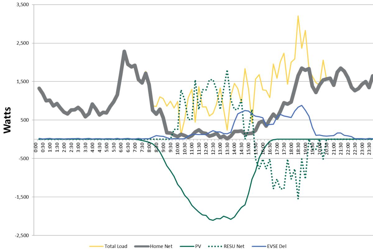
To illustrate the effect of the RESUs on the net load profiles of the ZNE Block homes, **Figure 14** presents the load profile of a single home on the CES Block for the same period. Since this home does not have a RESU to help regulate the homes' net demand, and since the solar PV generation was much greater than the home's energy demand, the net load was negative during much of the daytime hours.
