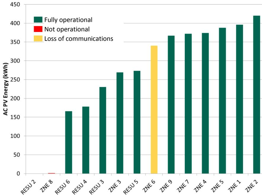
The ZNE Block has nine homes with solar PV arrays, each identically sized at 3.9 kW. Six of these produced over 350 kWh during the test period. The array at ZNE 6 produced less than 350 kWh, probably because it stopped operating late in the test. The array at ZNE 8 was never operational during the test period, and the array therefore produced no energy due to software issues. The array at ZNE 3 produced just 270 kWh. This is approximately 75% of the generation by the other arrays.
