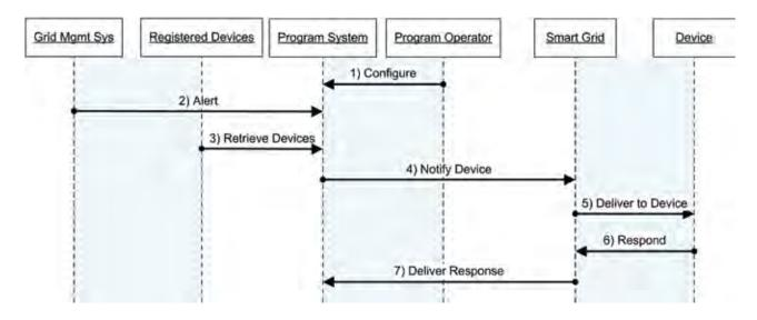
Figure 8 – Sequence Diagram for Usage (part of Customer Enablement in the Smart Grid)
