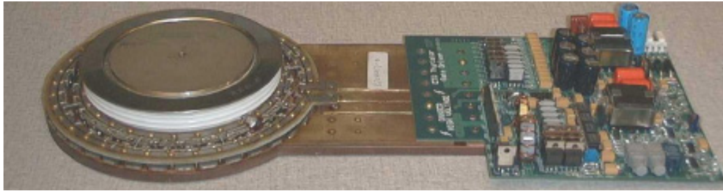
Fig. 4.10. 4000-A/4500-V ETO with the integrated gate driver [9].
