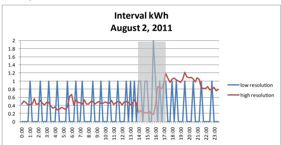
Figure 5-11. Relative Resolution of Decawatt-Hour and Kilowatt-Hour Meters
