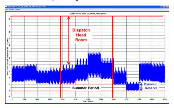
Figure 12: Transformer Loading Identifying Dispatch Headroom
