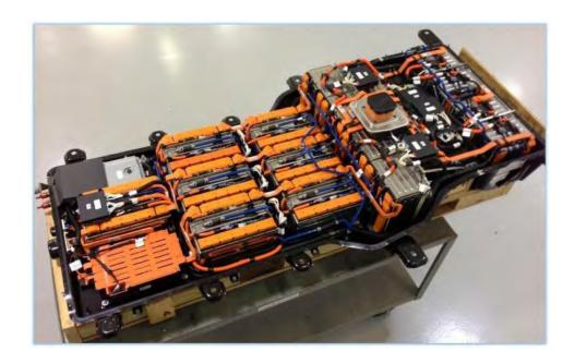
Figure 22: Open Fiat 500e Battery Pack Showing the Battery Modules
