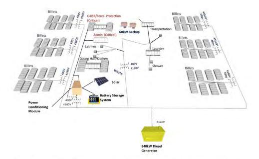
Figure 2: 550-person Battalion: 1 Generator with energy storage and alternative energy generation
