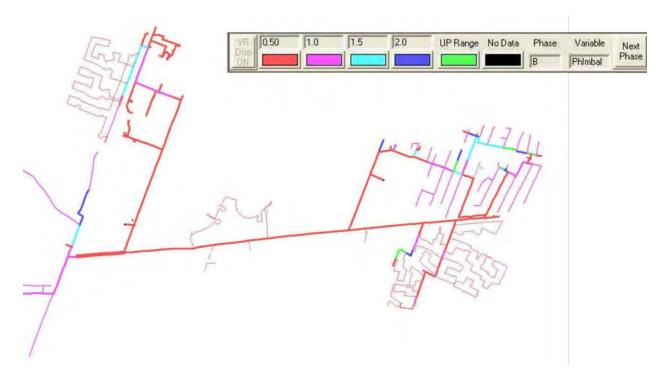
Figure 15: Circuit Model Identifying Phase Imbalance
