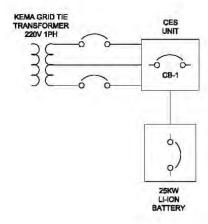
Fig 1. Test Set up with no load bank connected...
