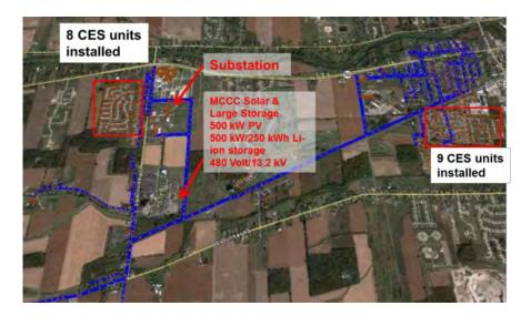
Figure 7: Location of Energy Storage Systems on the Trinity Circuit
