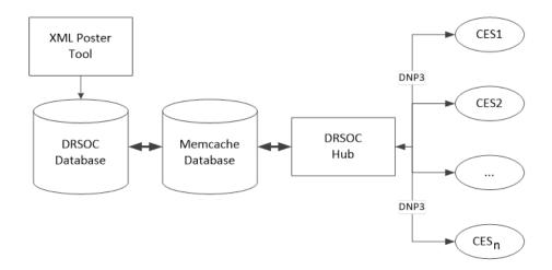
Figure 24: Schematic of CES Test Setup
