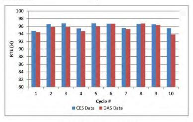
Figure 3. DC round trip efficiency
