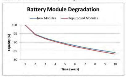
Figure 3-3 Battery Module Degradation for Peak-Shaving
