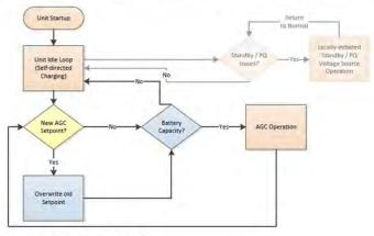
Figure 3-3 Frequency Regulation control logic
