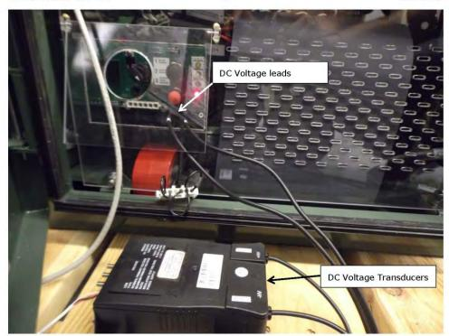
Figure 8. DC voltage measurement setup
