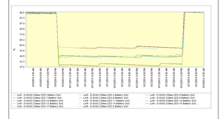
The graph below shows the kW set point (scale factor is 10,000) on the right axis and Battery SOC on left axis of CES-14. On June 10, 2014 at approximately 16:14, the unit was requested to export 25 kW. The unit did produce 25 kW for about 1 ½ hours, at which time it reached the Minimum Reserve Margin. At that time, despite the continued 25 kW set point, the unit retained a Battery SOC of approximately 40%.
