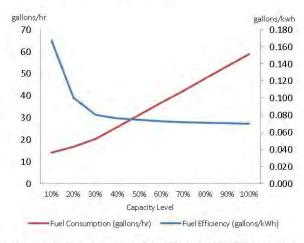
Figure 4: Fuel consumption and efficiency of 840 kW generator
