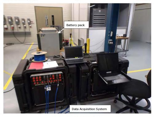
Figure 10. Data acquisition system
