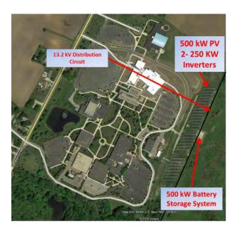
Figure 8: Location of 500 kW PV and Storage at MCCC
