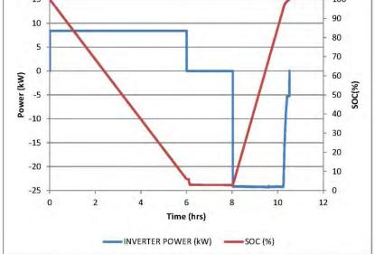
Figure 4d. Second peak shaving profile test at 8.4 kW discharge
