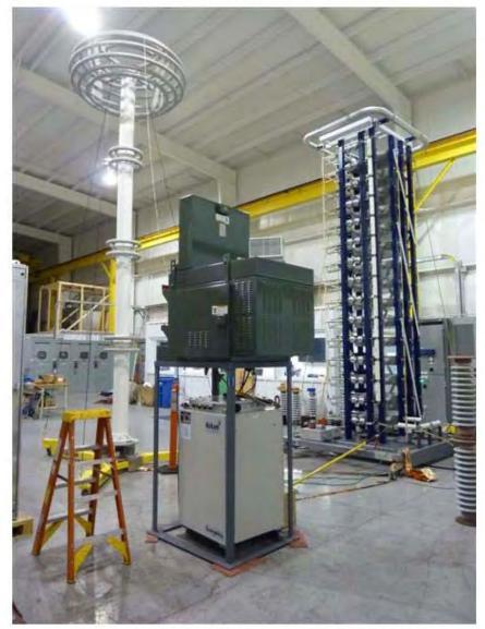
Set up for BIL test. CES unit and battery on test stand. KEMA Impulse generator is the blue rack to the right and white voltage divider on the left.
