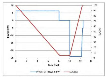
Figure 4a. First peak shaving profile test at 6.3 kW discharge
