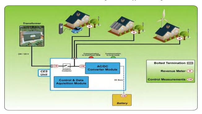
Figure 3: CES Application Diagram
