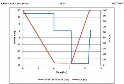
Figure 4f. Second peak shaving profile test at 12.6 kW discharge
