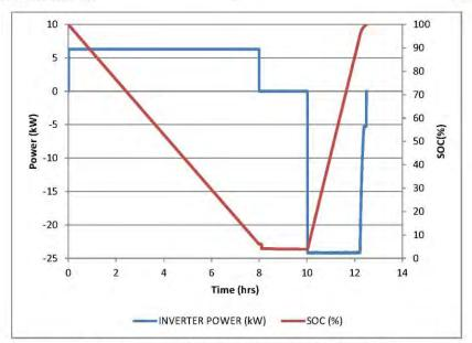
Figure 4b. Second peak shaving profile test at 6.3 kW discharge
