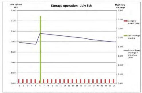
Figure 4-2 Net Storage Dispatch and State-of-Charge for MISO Market Case with New Battery Modules – July  $\mathbf{5}^{\text{th}}$
