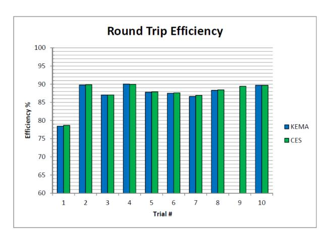
Figure 27: CES AC Round Trip Efficiency
