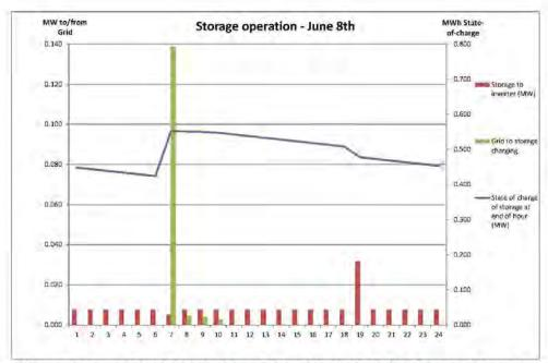
Figure 4-4 Net Storage Dispatch and State-of-Charge for MISO Market Case with New Battery Modules - June 8<sup>th</sup>
