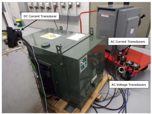
Figure 9. DC current and AC current and voltage measurement setup
