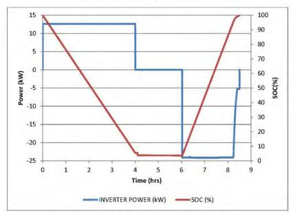
Figure 4e. First peak shaving profile test at 12.6 kW discharge
