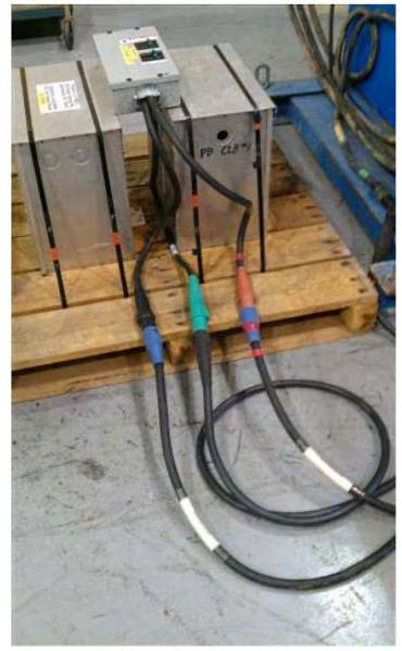
Capacitive load bank connections
