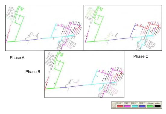
Figure 13: Circuit Model Identifying Phase Voltage for CES Placement
