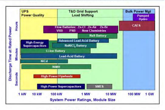
Figure 3: Positioning of Energy Storage Technologies
