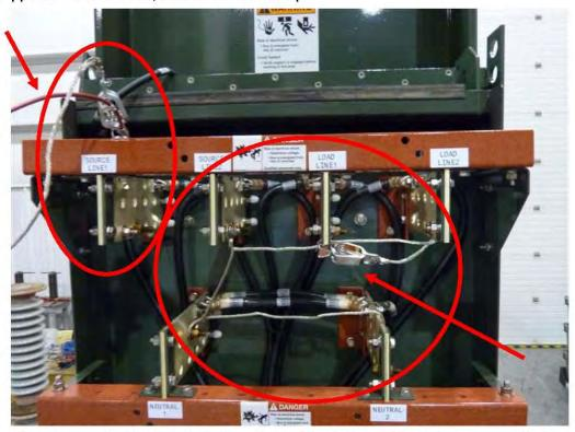
Typical connection for BIL test. CES source line 1 tied to the red high voltage clip and all other terminals to ground through the un-insulated stranded wire. The second clip attached to the CES source line 1 is for the voltage divider.
