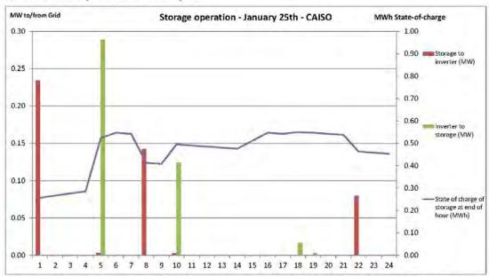
Figure 4-11 Net Storage Dispatch and State-of-Charge for CAISO Market Case with New Battery Modules - January  $25^{\rm th}$
