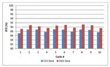
Figure 2. AC round trip efficiency
