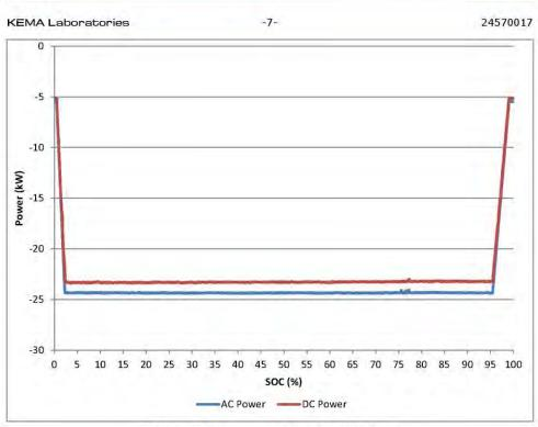
Figure 1. Charge power vs. battery state of charge
