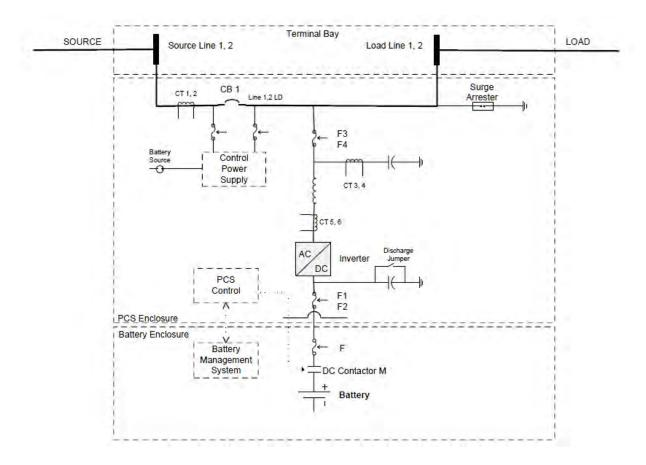
Figure 4: CES Electrical One Line Diagram
