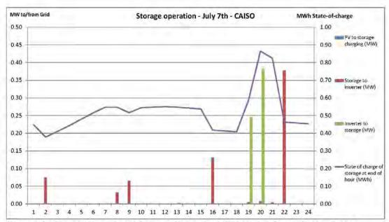
Figure 4-9 Storage Dispatch and State-of-Charge for CAISO Market Case with New Battery Modules - July  $7^{\text{th}}$
