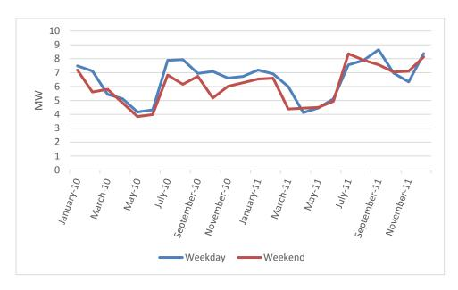
Figure 9-2 Monthly Average Loads at Monolith Substation
