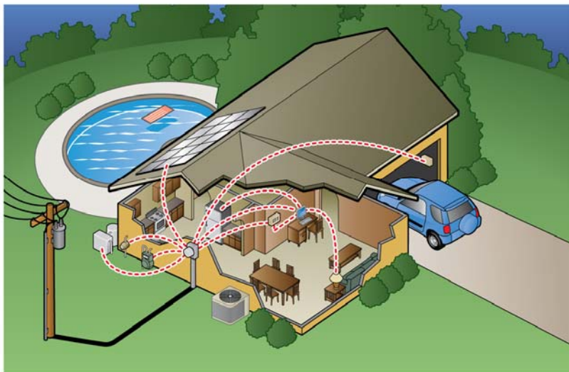
Figure III-1. Illustration of AMI and home-area-networks
