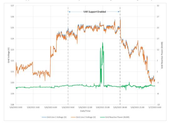
Figure 142: VAR Support Test 1 Performed on May 6, 2015 and Using an Over Voltage Multiplier of 104.0%
