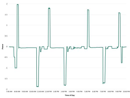
Figure 168: DBESS Charge/Discharge Profile (October 24, 2014)
