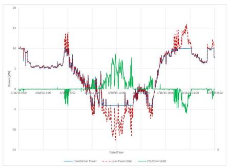
Figure 4: CES Load Limiting Behavior
