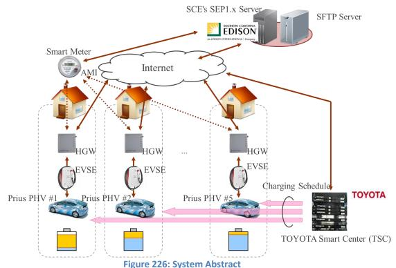
The system comprise of Toyota Smart Center, Home Gateway (HGW), EVSE, smart meter, the utility's demand response serve and SFTP server.
