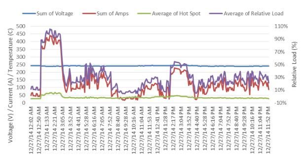
**Figure 83** presents the 2-day plot of transformer load versus temperature, indicating how transformer temperatures rise and cool based on load. The spring months resulted in a more gradual warm up of the transformer temperature due to the increased PV generation and higher associated current. Transformer temperatures drop to 30 degrees Celsius around 7:00 am daily. The temperature then begins a slow rise as PV generation increases, spiking suddenly when RESU operation begins at 2:00 pm.
