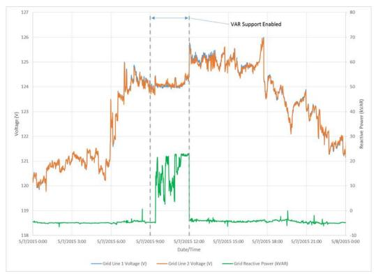
Figure 143: VAR Support Test 1 Performed on May 7, 2015, Using an Over Voltage Multiplier of 103.0%
