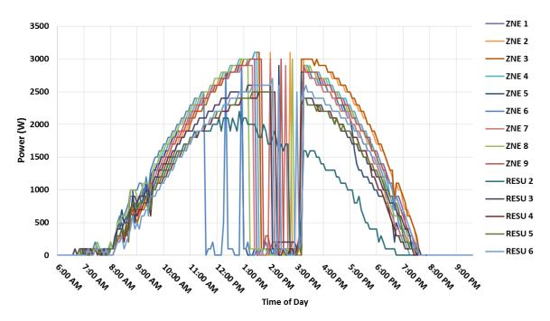
Figure 69: Solar PV Generation Output (July 8, 2014)
