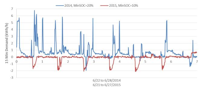
Figure 114: RESU 5 Demand Comparison under Two PV Capture Tests
