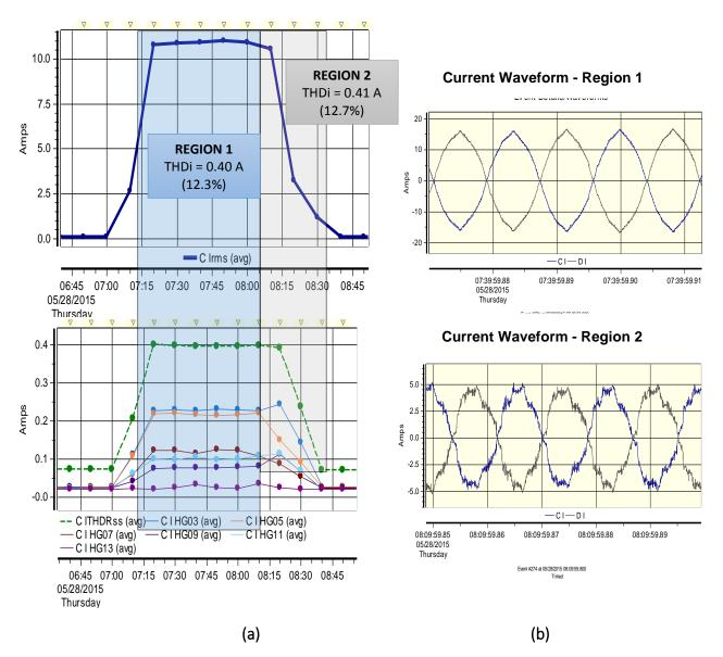
Figure 198: (a) Toyota Prius charging current profile (b) Current Waveforms
