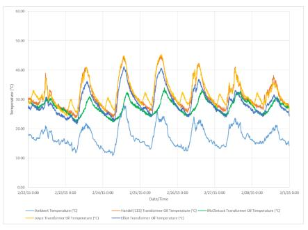
Figure 134: Transformer Oil Temperatures between February 22 and March 1, 2015
