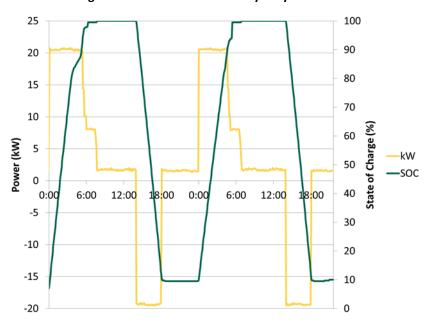
Figure 9: Solar Car Shade Battery Only Load Shift
