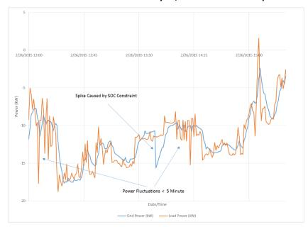
Figure 140: Grid and Load Power on February 26, 2015 between 12:00 pm and 3:30 pm
