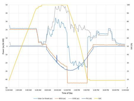
Figure 10: Solar Car Shade Whole System Load Shift
