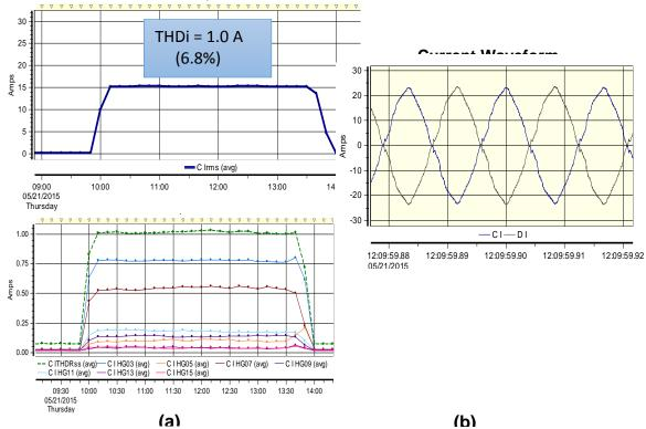
Figure 200: (a) Chevy Volt charging current profile (b) Current Waveform
