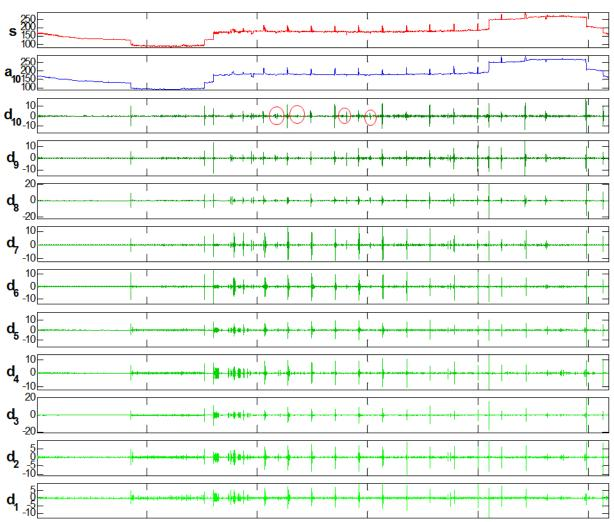
Figure 174: Wavelet Decomposition of the Current Signal
