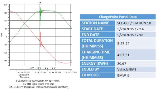
Figure 195: Impulsive transient event at EVSE 8
