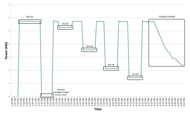
This second round of commissioning tests confirmed the results of the first round, that an EVSE's ability to perform duty cycle DR events is constrained by the charging capacity of the EVSE and the vehicle's onboard charger. Chapter 5 discusses this finding in more detail.
