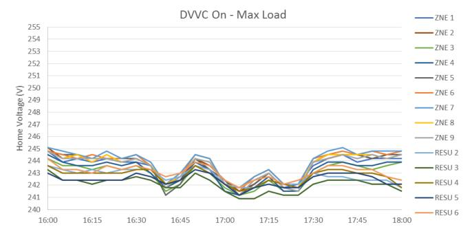
**Figure 91** and **Figure 92** illustrate the local home voltages with little to no PV generation and minimal loading. With DVVC off and DVVC on, a lower overall voltage is still observable despite a lack of PV generation. On the latter portion of the DVVC off portion, local voltages rise as the sun begins to rise around 6:15 am. The impact of VARs can be seen faintly as a small dip in the general voltage trend between 5:20, and 5:41 am.
