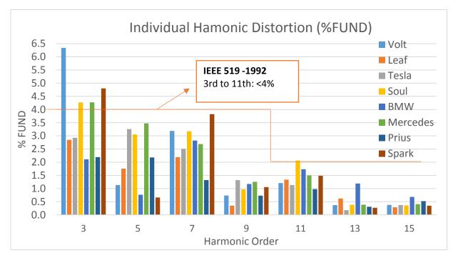
Figure 201: Comparison: Individual Harmonic Input (% FUND) for different EV models
