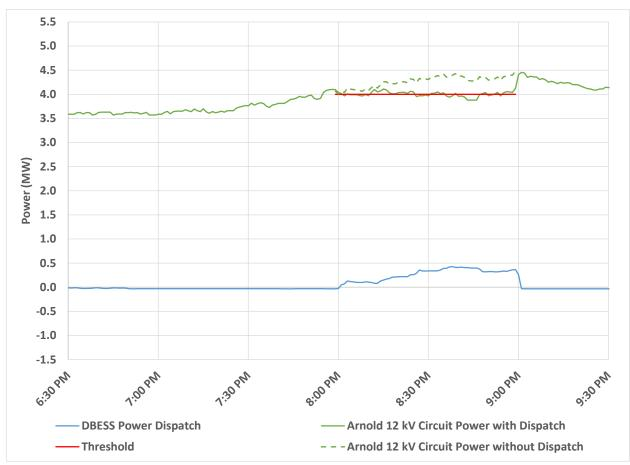
Figure 164: DBESS Peak Load Shaving/Feeder Relief
