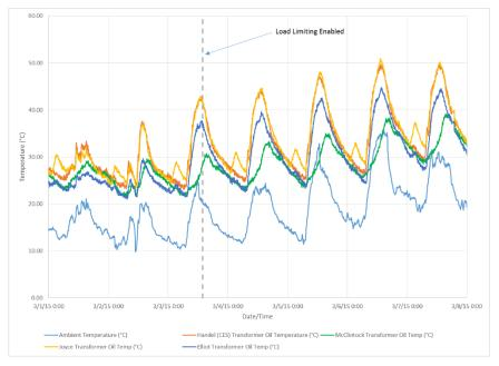
Based on **Figure 134** and **Figure 135**, the oil temperatures of the ZNE and CES Block transformers are generally within 2°C of each other. The only exception occurs between 1:00 am and 3:00 am. The RESUs in the homes serviced by the ZNE Block transformer were running a load shifting profile and the ZNE Block Transformer was at more than 70% its capacity during those hours. As a result, a temperature spike could be observed during those hours. Other than the
