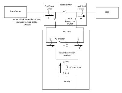
To allow the CES to service the neighborhood, the CES's load connection switch would need to be closed and the bypass switch opened. **Figure 124** shows the electrical configuration of the CES. The CES would then be able to supply power to the homes in the neighborhood in the event of a grid outage. To avoid any unexpected issues that would arise in the actual islanding test, the ISGD team monitored the load characteristics of the neighborhood and the CES's behavior during grid events.
