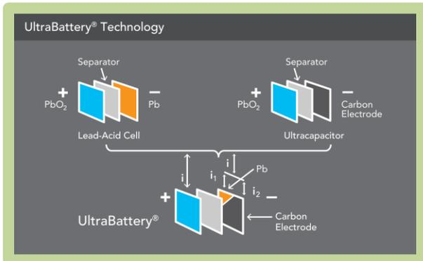
Figure 3. Lead-acid cell (top left), ultracapacitor (top right), UltraBattery® (bottom). Courtesy of East Penn.
