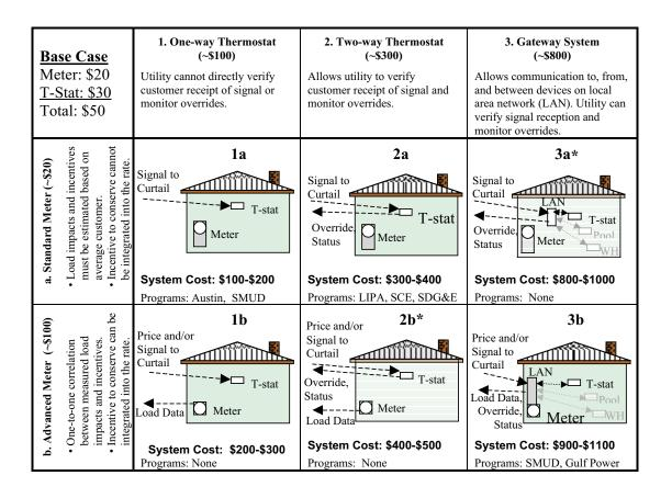
Figure 3-j. Communicating thermostat hardware configurations options and cost estimates.
