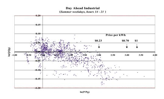
Figure 3-1. Demand response of industrial Day-Ahead customers in Georgia Power's RTP program. Customers have loads greater than 5 MW; 25% of the customers have on-site generation.
