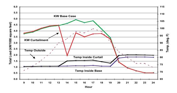
Figure 3-e. DOE-2 Simulation of a hypothetical medium-sized office on a hot day (max.  $100^{\circ}$  F) in Sacramento. The curtailment case assumed a  $4^{\circ}$  F thermostat set-up and one-third lighting reduction. Curtailment was initiated at 1 p.m. and concluded at 5 p.m. Impacts per 1,000 ft<sup>2</sup> were: Average Hourly Savings: 1.5 kW (1-5 p.m.); First Hour Savings (1 p.m.) = 2.7 kW; Total Savings Daily 6.1 kWh.
