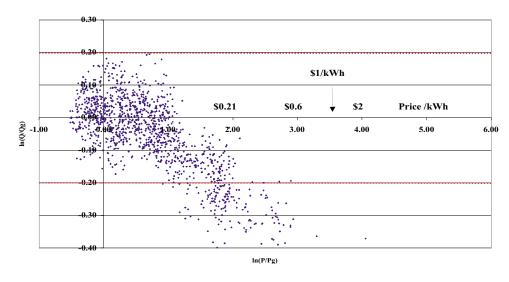
Figure 3-k. Demand response of large industrial Hour-Ahead customers in Georgia Power's RTP program. Scales are logarithmic. We have added on the x-axis a few price levels in \$ per kWh.
