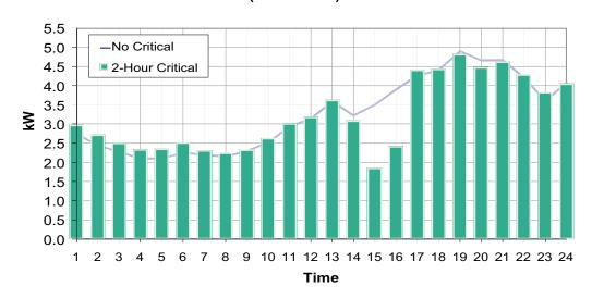
Figure 3-i. Average Load and Load Reduction in Gulf Power CPP program. The TOU rate (11 a.m. to 8 p.m.) was 9.3 ¢/kWh. The 1- and 2-hour CPP was 29 ¢/kWh, an extra 20 ¢/kWh. The 2-hour CPP dispatch was at hours was at hours 15 and 16.
