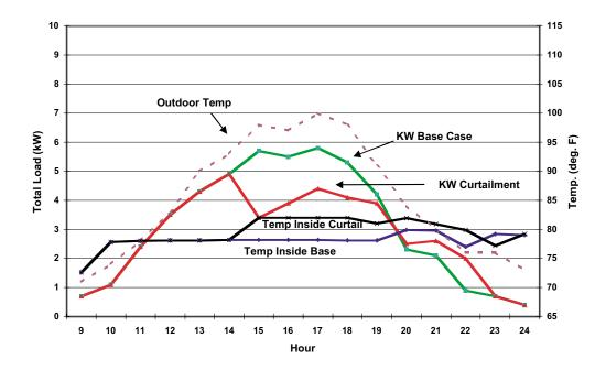
Figure 3-g. Simulation (DOE-2) of a hypothetical Single-Family Residence Hot Day (Max. 100°F) in Sacramento. Curtailment case is a thermostat offset of 4°F from 2 p.m. to 6 p.m. Curtailment savings of: Avg. kW (2-6 p.m.) = 1.6; First Hour kW (2 p.m.) = 2.3; Total from 2 p.m. to 6 p.m. = 6.4 kWh however, daily savings equals = 5.0 kWh due to rebound effect.
