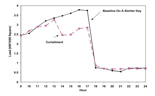
Figure 3-f. Actual measured air conditioning load in SMUD office building. Curtailment involved a thermostat set-up of  $4^{\circ}$  F from 1 p.m. to 5 p.m. Lights were dimmed. The load after hour 18 is from fans which run continuously and cool the building overnight.
