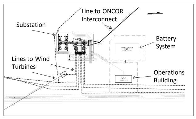
Figure 2-7 Location of Dynamic Power Resource in Relation to Substation and Operations Building
