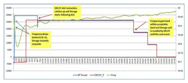
Figure 6-18 Illustration of BESS Arresting Extreme Frequency Deviation (Source: Xtreme Power)
