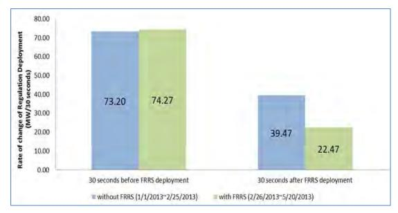
Figure 6-17 Rate of Change of Regulation Deployment (MW/30 seconds) (Source: ERCOT)
