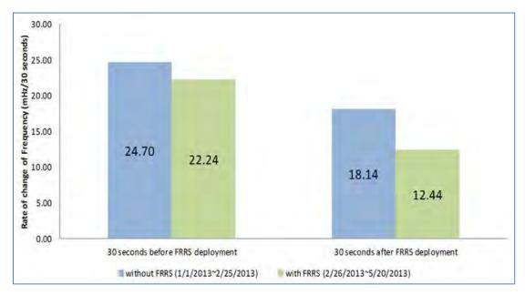
Figure 6-16 Rate of Change of Frequency (mHz/30 seconds) (Source: ERCOT)
