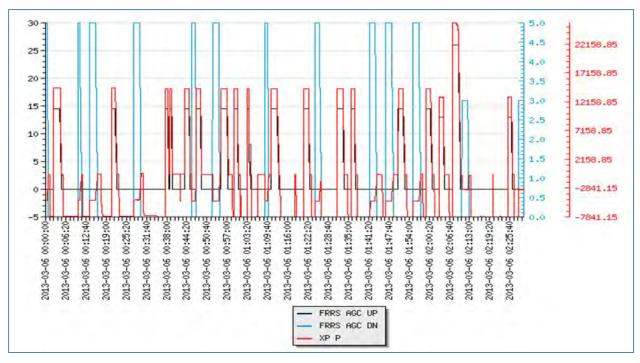
Figure 6-27 Response of BESS (in red) to ERCOT Regulation Signals, March 6, 2013 (Source: Xtreme Power)
