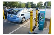
(c) Plug-in Hybrid/Electric Vehicle Charging Station
