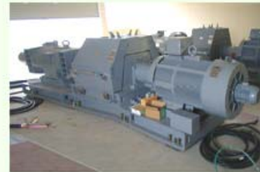
150kW rotating type generator (simulates WP, Co-generation)
