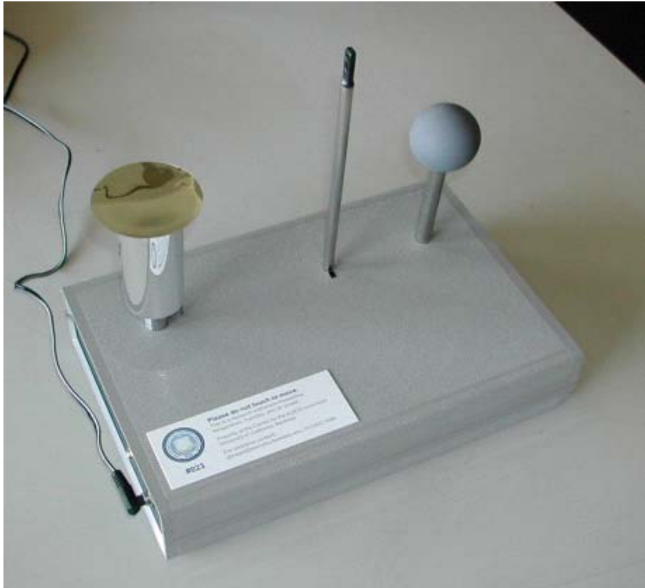
Figure 3. Indoor climate monitor with (from left to right): shielded dry bulb sensor, anemometer (air speed sensor), and globe temperature sensor
