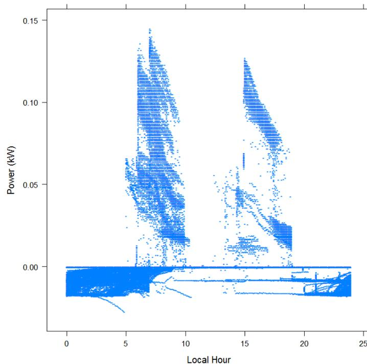
**Figure 8.14.** Sum Power Generation of Two 1 kW Energy Storage Modules versus Local Pacific Time. Benton PUD responded that positive power indicated charging the batteries, but that might be incorrect for these 1 kW modules.
