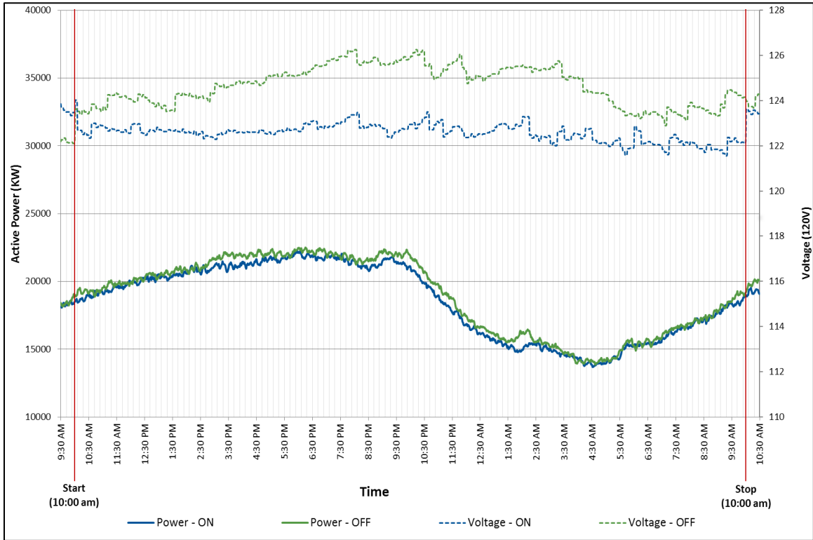
Figure 3-39: TF #7/8 Active Power & Voltage Comparison (07/15 – 07/16)
