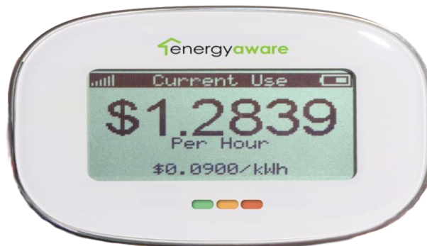
Figure 2-4: In Home Display Used in SPO Pilot
